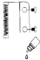
To keep the device in optimum condition, the blades should be lubricated after a few cuts.
