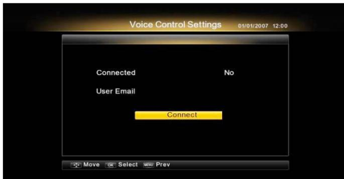
Press the **OK** key on Connect, the screen will appear the dialog box of INFORMATION: to enable standby mode select YES; a window will appear to enter the previously created association code: use the numeric buttons on the remote control.
